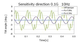
Cut-off frequency and Time constant against Damper setting are shown the below table. It is possible to choose the best Damper time constant by operating speed and vibration condition.
